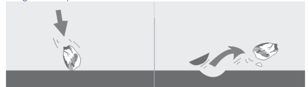
Abrasive particle striking non-elastic metal surface. Conversion of kinetic energy into impact, friction and noise.
