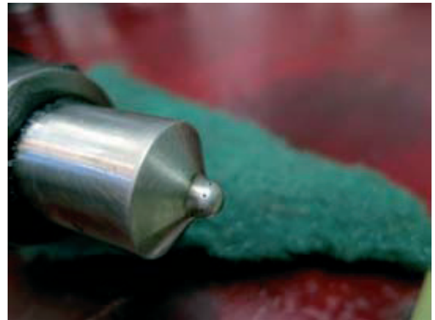
Nozzle condition before cleaning & after cleaning with a nylon sponge.
