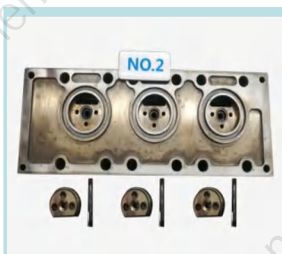
Injection control block
