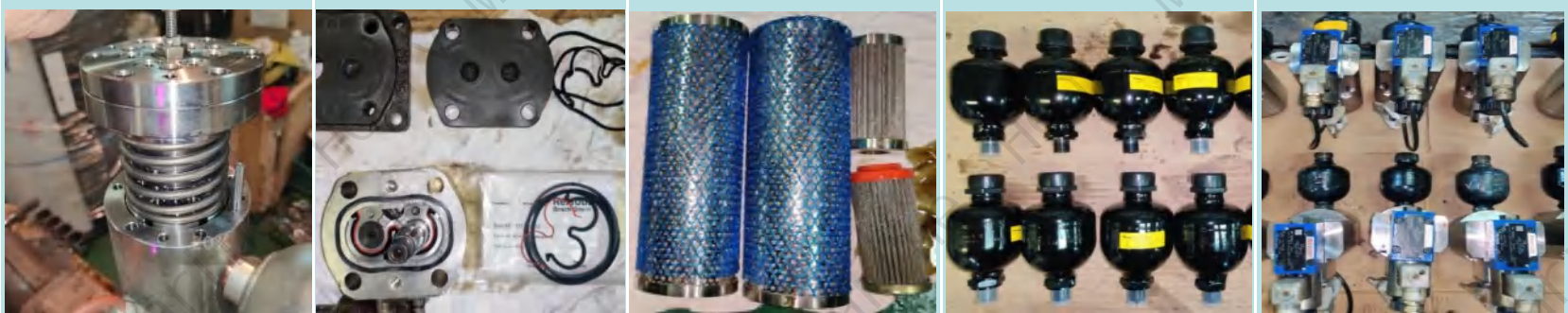
Overhaul cylinder lubricating system with spare parts
