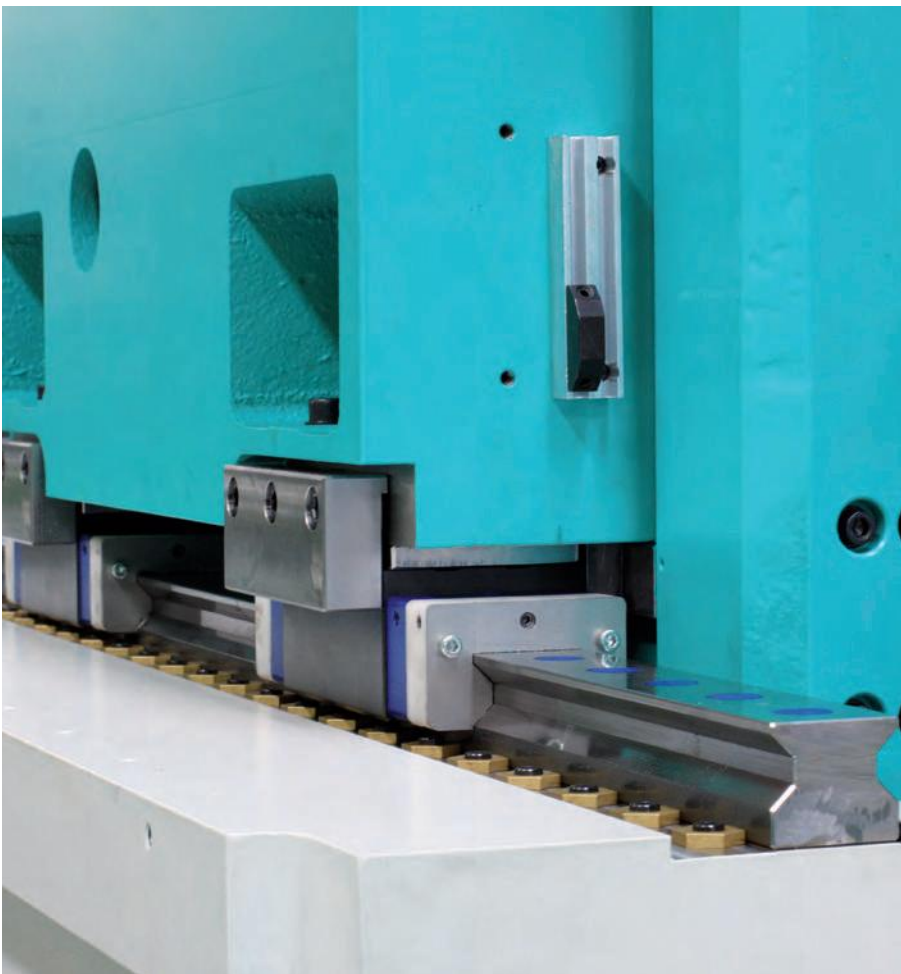
Horizontal and vertical axes on Rosa Ermando SpA grinding machine.
