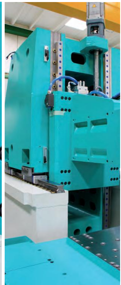
Horizontal and vertical axes on Rosa Ermando SpA grinding machine.
